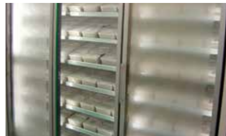
Specially-treated panes enable the middle door to remain fog-free, in comparison with non-treated doors on the left and right, all photographed shortly after opening in the trial lab.
