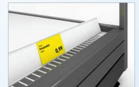
The new return air grid also acting as an area for pricing and product stop, preventing obstructions of the air flow.
